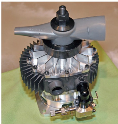
← Mr. Takumi Muroki, a member of the first RE development team, the so-called RE 47 Ronin, showed us a small single-rotor air-cooled RE for aircraft, which may be used for unmanned aerial vehicles somewhere. This is an example of how RE is being used in places we do not know.
